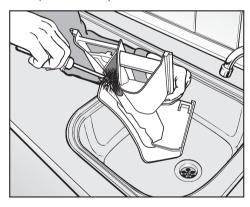
Clean the fabric softener channel with warm water and a brush. If liquid starch is used often, the siphon and fabric softener channel will need to be thoroughly cleaned. Liquid starch can cause a build-up and clogging.
